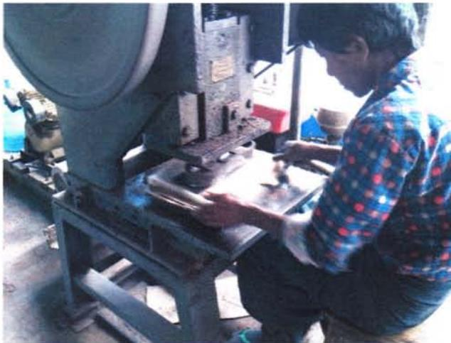
Figure (6) leather cutting mold
